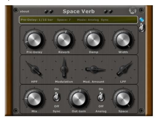
Space ship stereo reverb with pre-delay (up to 1 second or from 1/32 bar to 2 bars, if in sync) with automated feedback (feedback can be turned off), exclusive reverb modulation stage (1 or 2 LFOs), 6 or 12 dB/octave LP and HP filters, analog emulation with bypass switch, 7 different spaces (from dark to bright), output amplifier with mix knob and internal limiter, master bypass switch, dual spider eyes meters for input and output level, LCD display, back view with extra control switches.
