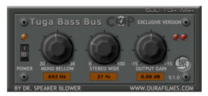
Bass Bus processor with transparent 6dB crossover filter acting as "mono bellow/stereo above" and stereo wideness control (does not affect the mono signal).
