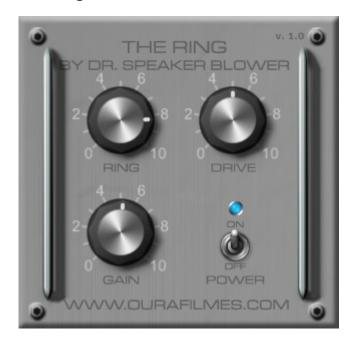
The Ring – Ring modulation effect. Custom made for a friend, under his supervision. It outputs the difference (frequencies) between the left and right channels. Use the Ring knob as a dry/wet knob and warm it in the valve drive section. Killer SFX creator on a send BUS!
