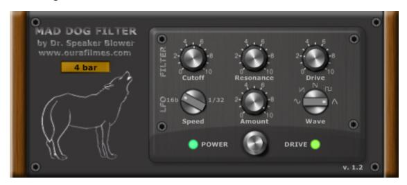
Exclusive design, liquid 24 dB LP filter based in the classic Moog ladder filter with post filter drive section, Ifo with sync rates only and classic waveforms, LCD display, led style drive amount meter.
