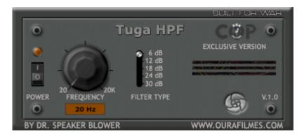
Transparent hi-pass filter (20 Hz to 20 KHz): from 6dB/octave to 30 dB/octave.
